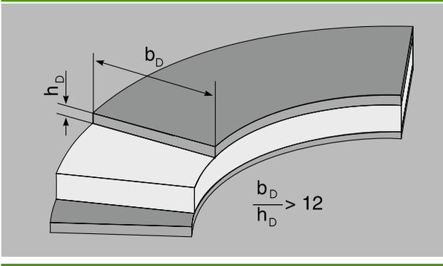
RivaTherm-Compact consists of a stainless steel sheet as carrier material and a 0.5 mm graphite foil glued on both sides as sealing material. All common stainless steel qualities are available. Sheet metal carriers made of other metallic materials with a smooth, scale-free surface are also possible.
