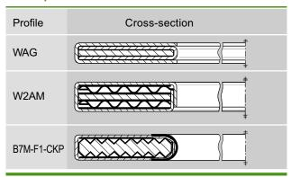
In **Profile W2AM** gaskets, the inner steel ring is layered with corrugated gaskets with graphite layers and then coated with fibreglass. The gaskets are generally impregnated.
