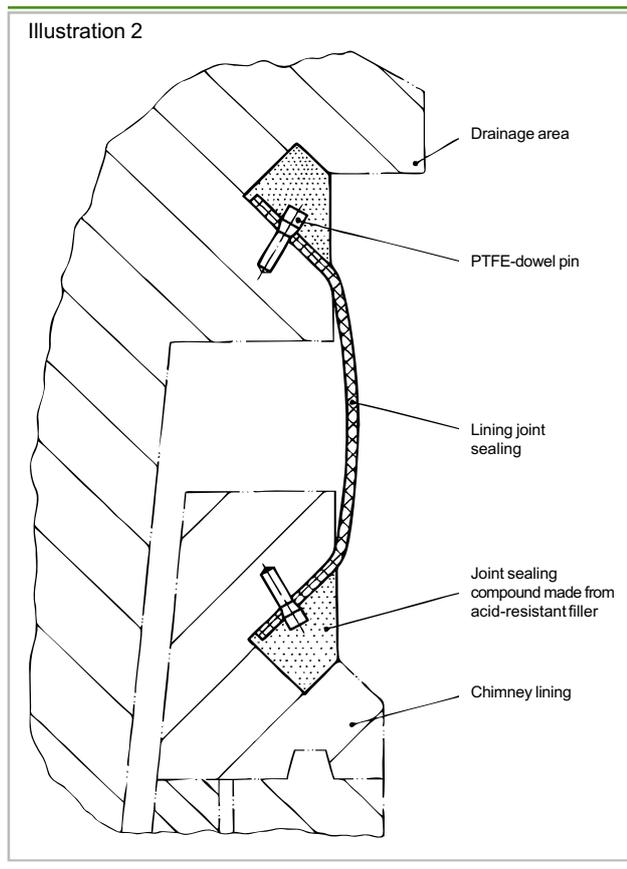
Installation takes place in two directions towards the joint. The connection procedure stops a few metres away from the joint so that the sealing strip can be trimmed to its finished dimension. The joint is produced using a portable hydraulic vulcanising press. Any remaining gaps are then filled with a self-vulcanising highly viscous fluor rubber surface.
